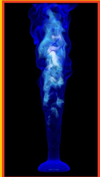
Three-dimensional rendering of hydroxyl radical in a direct numerical simulation of a highly turbulent premixed jet flame. Simulation by Haiou Wang and Evatt Hawkes, University of New South Wales; rendering by Hongfeng Yu, University of Nebraska-Lincoln.
