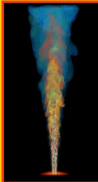
Three-dimensional rendering of vorticity magnitude in a direct numerical simulation of a highly turbulent premixed jet flame. Simulation by Haiou Wang and Evatt Hawkes, University of New South Wales; rendering by Hongfeng Yu, University of Nebraska-Lincoln
