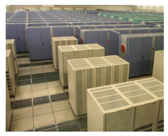
supercomputer to use the classical vector processing design approach. It stayed on the Top500 for two years until the IBM Blue Gene appeared.
